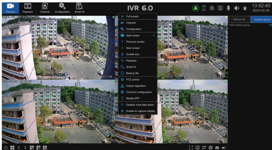
Turn off the sound and light alarm: Click to enter the menu, user can select the channel one key to turn off the sound and light alarm of IPC, as shown in the following figure.
