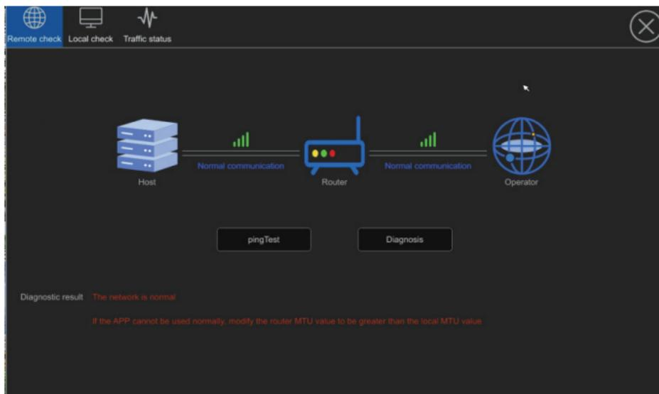
**Remote diagnosis:** Displays the network connection status between the IVR, router, and carrier.
