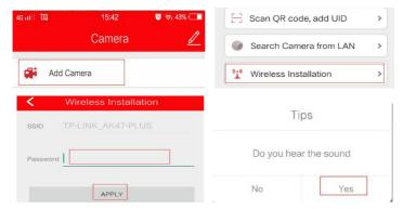
(4), Turn the phone sound up and come close to the camera. It will show camera is connected after the right configuration of WIFI, camera connection is successful, wait about 100 seconds to jump to a camera list, click the ID number, can modify the camera name, then click the top right corner, the real-time video can be seen by clicking camera name in the home page, as below shows:
